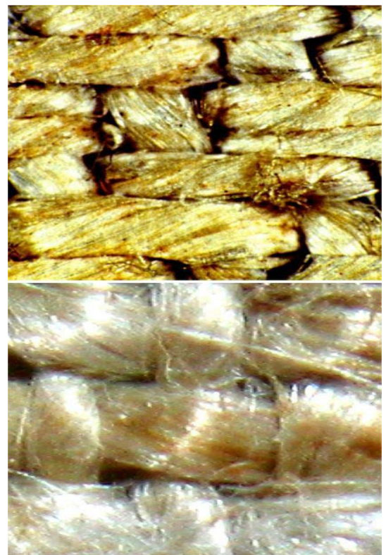
Figure 4: Striations (E8) of the image-threads: on the top, detail of the TS eye (M. Evans ME20, ©STERA Inc. kind permission of B. Schwartz), where also a crevice appears; on the bottom, for comparison striations obtained with Corona Discharge (CD) experiments.
