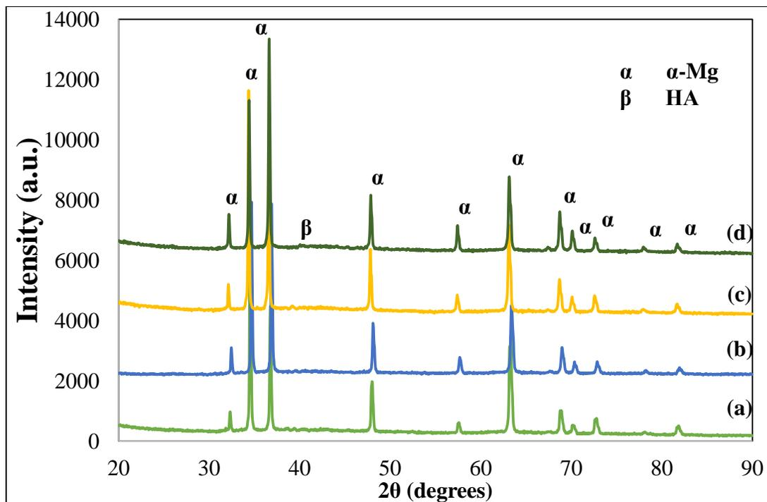
Fig. 1 XRD patterns of Mg-Zn/HA being milled for (a) 2 hours, (b) 4 hours, (c) 6 hours and (d) 8 hours
