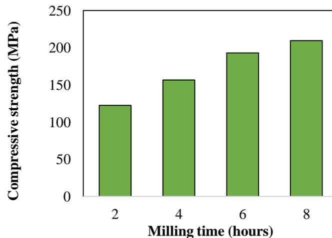
**Fig. 4** The ultimate compressive strength of Mg-Zn/HA composite milled under various milling time
