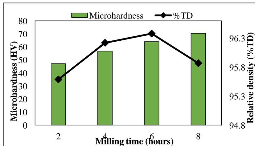
**Fig. 3** Plot of microhardness and densification of Mg-Zn/HA composite being milled under various milling time
