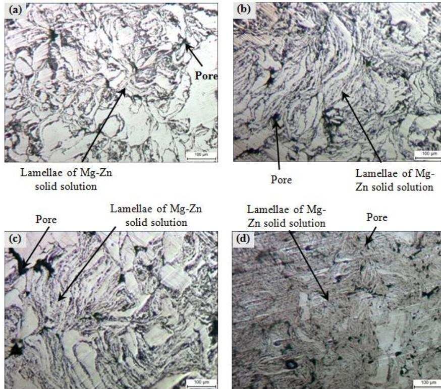
**Fig. 2** Micrographs of Mg-Zn/HA composite fabricated by planetary mill for (a) 2 hours, (b) 4 hours, (c) 6 hours and (d) 8 hours
