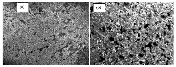
Fig. 2 SEM morphology for 55B glass (a) Before immersion and (b) After immersion for 16 weeks
