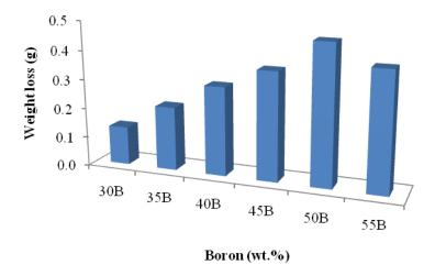
Fig. 3 The weight loss of different contents of boron oxide (wt.%)
