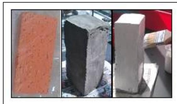
**Fig. 1** (a) Ordinary red brick with standard size of  $8 \times 4 \text{ cm}^3$ , (b) Fully coated brick with concrete plaster before coating process and (c) Coating materials was applied on the surface of concrete plaster
