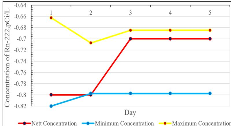
**Fig. 6** Nett, minimum and maximum of  $^{222}\text{Rn}$  concentrations in red brick layered with plaster and coated with coating C
