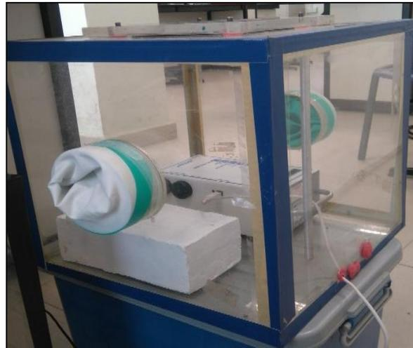
**Fig. 2** Measurement of <sup>222</sup>Rn concentration using Radon Sentinel 1030 in a close perspex box
