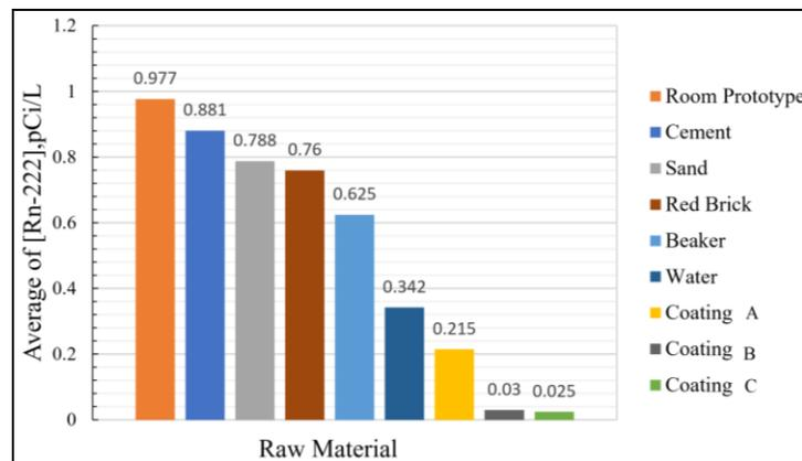
**Fig. 3** Average of <sup>222</sup>Rn concentrations for raw materials and empty prototype room
