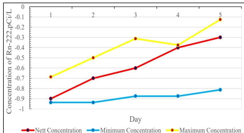
**Fig. 5** Nett, minimum and maximum of  $^{222}\text{Rn}$  concentrations in red brick layered with plaster and coated with coating B
