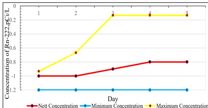
**Fig. 4** Nett, minimum and maximum of  $^{222}\text{Rn}$  concentrations in red brick layered with plaster and coated with coating A
