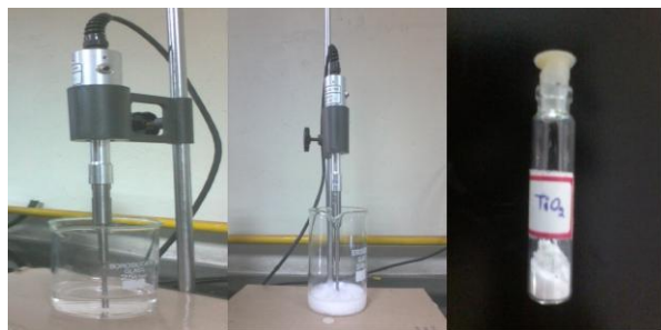
Fig.1: 1(a) NaOH solution, 1(b) drop wise addition of Tetra isopropoxide Titanate 1(c) Final TiO_2 product Synthesized by Sonochemical method.
