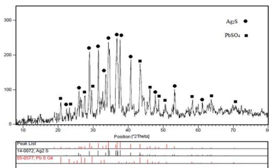
Fig. 1: XRD patterns of  $\text{Ag}_2\text{S}/\text{PbSO}_4$  Nanocomposites.
