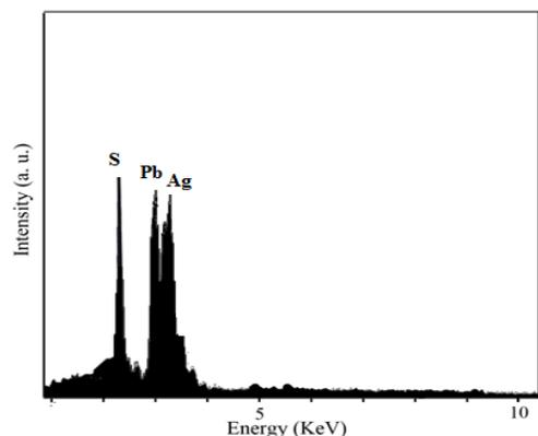
**Fig. 5: EDS pattern of  $\text{Ag}_2\text{S}/\text{PbSO}_4$  nanocomposites (sample no.A2).**
