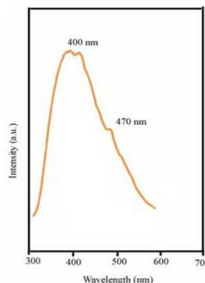
Fig. 4: Room temperature PL spectra of  $\text{Ag}_2\text{S}/\text{PbSO}_4$  nanocomposites sample no. A2
