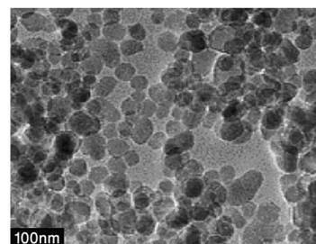
Fig. 3: TEM image of  $\text{Ag}_2\text{S}/\text{PbSO}_4$  nanocomposites (A2).
