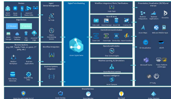
Figure 1: Azure Digital Twins reference architecture (source: Microsoft).
