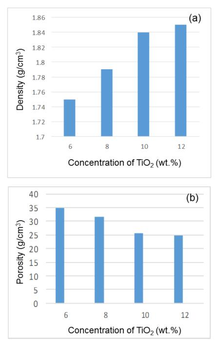
Fig. 2 (a) Density and (b) Porosity of MLCM at different concentration of TiO<sub>2</sub>
