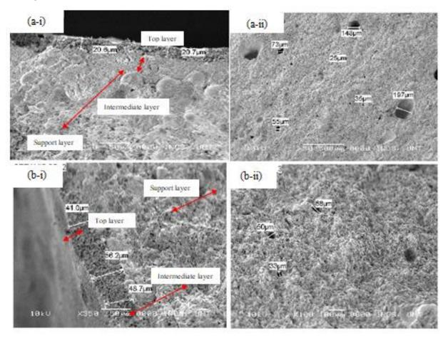
Fig. 3 Morphology of MLCM (a) 6 wt.% TiO<sub>2</sub> and (b) 12 wt.% TiO<sub>2</sub>
