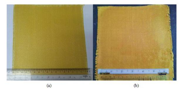
Fig. 3 Laminated composite (a) Kevlar 29/Epoxy composite and (b) Kevlar 29/Epoxy/Cellulose micro/nanocomposite
