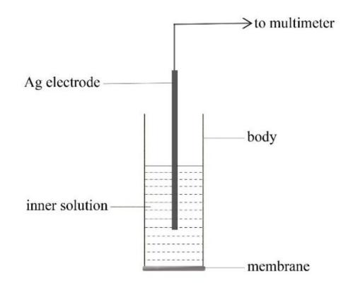
Fig. 1 Ion Selective Electrode (ISE)
