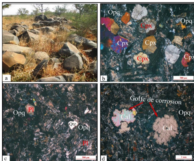
Figure 3: Field photograph showing the outcrop of a dyke at Toufeultréné and photomicrograph attesting to the magmatic texture. a: Outcrop in the form of balls and blocks of dolerite dykes with pyrite and calcite at Teufoultréné; b: Intergranular to granophyre texture. Note the abundance of opaque minerals and the presence of quartz in the dolerite with pyrite and calcite in LPA (sample TERM4); c: Note the presence of clinopyroxene phenocrysts and opaque minerals (TESM4 thin section, LPA); d: Calcite crystals with corrosion gulfs in dolerite with pyrite and calcite in LPA (sample TEIM3). Opq: opaque, Cpx: clinopyroxene, Pl: plagioclase, Qtz: quartz and Cal: calcite.
