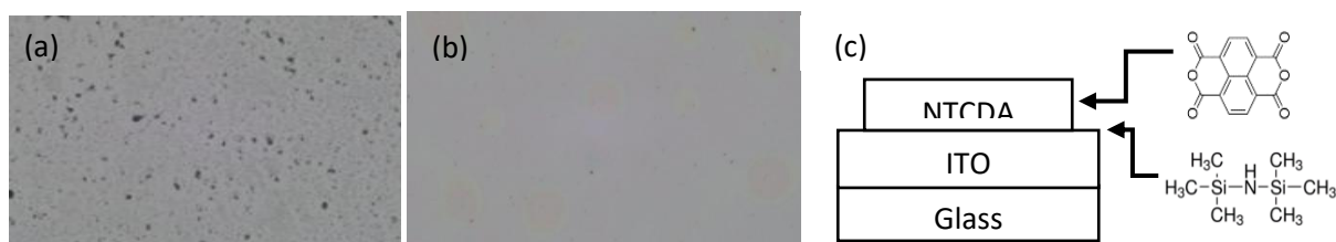
Fig. 1 The photomicrogram of NTCDA film after (a) 120 H, (b) 240 H of continuous stirring at temperature 100 °C. The images were taken under 10x magnification and (c) Sample structure of glass/ITO thin film/NTCDA film. The HMDS are deposited as SAMs between the electrode and organic layer
