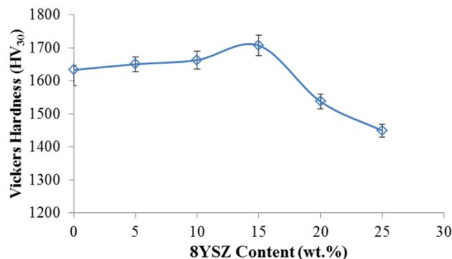
Fig. 1 Vickers hardness values of HIP sintering as a function of 8YSZ content
