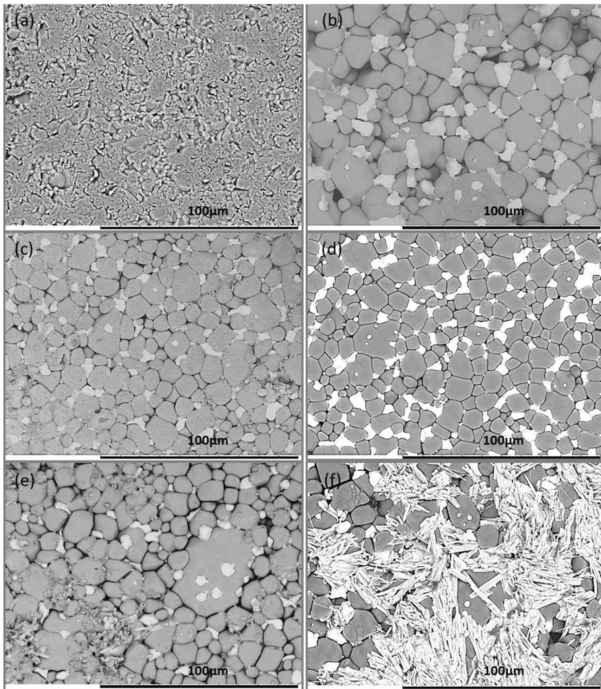
**Fig. 3** Scanning electron micrographs of  $Al_2O_3$  ceramics with (a) 0 wt.% of 8YSZ, (b) 5 wt.% of 8YSZ, (c) 10 wt.% of 8YSZ, (d) 15 wt.% of 8YSZ, (e) 20 wt.% of 8YSZ and (f) 25 wt.% of 8YSZ, at 1K magnification. Light grains: zirconia; dark grains: alumina
