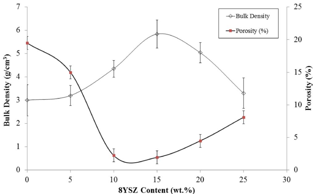
**Fig.4** Results of bulk density and percentage of porosity via HIP sintering technique
