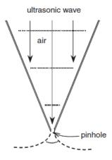
**Fig. 2** The propagation of ultrasonic signal in the cone
