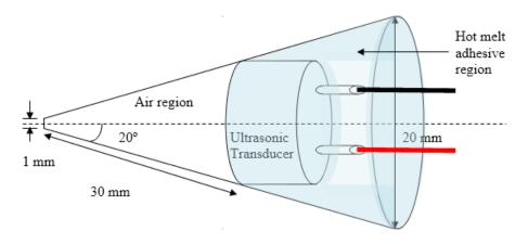
Fig. 1 The dimensions of the cone. The red and black lines are the wires to the ultrasonic transducer
