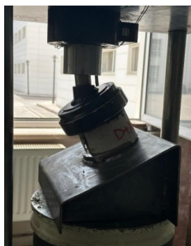
Figure 8: Loading the inclined device.
