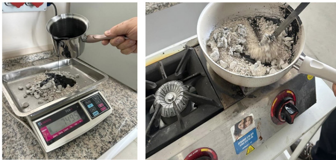
Figures 5 and 6: Weighing and heating of aggregate and bitumen materials.
