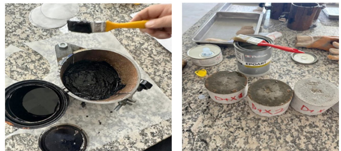
Figure 10: Aggregates added to surfaces with emulsion application / Application of epoxy to concrete surface.
