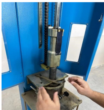
Figure 7: Compaction with Marshall hammer.
