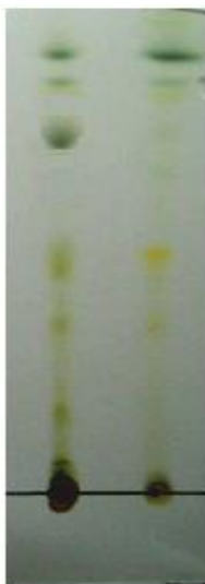
Fig. 6: TLC Chromatogram of Crateva adansonii bark extracts (Lane 1- Methanolic bark extract, Lane 2- Chloroform bark extract).
