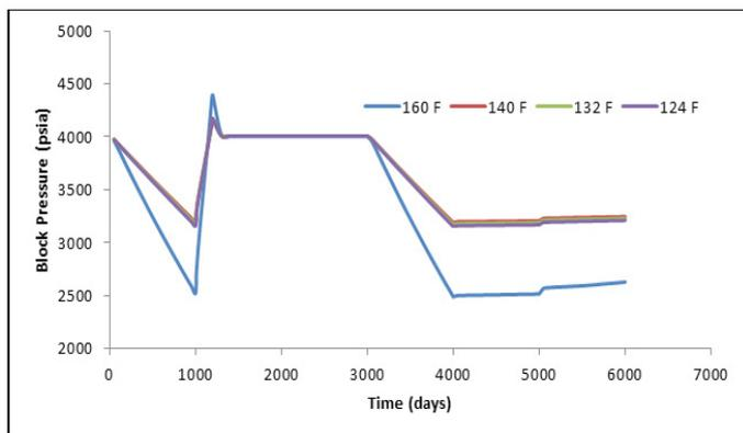
**Figure 14:** Block pressure vs time at different reservoir temperatures (injector well).
