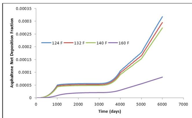
**Figure 15:** Asphaltene net deposition fraction vs time at different reservoir temperatures (producer well).
