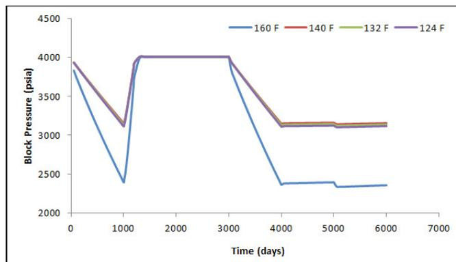
**Figure 16:** Block pressure vs time at different reservoir temperatures (producer well).
