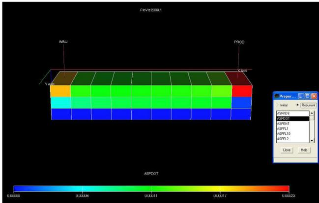
Figure 6: Asphaltene net deposition volume fraction.
