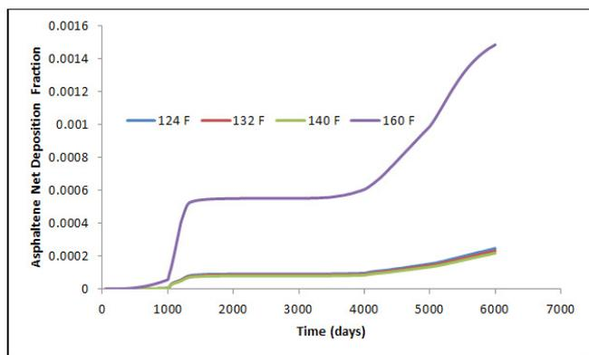
**Figure 13:** Asphaltene net deposition fraction vs time at different reservoir temperatures (injector well).
