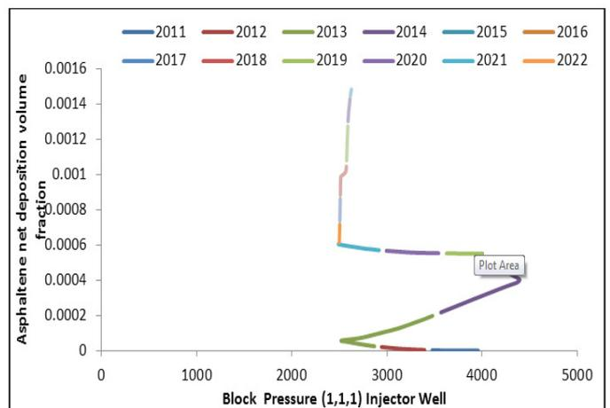
**Figure 4:** Asphaltene net deposition volume fraction vs block pressure (Injection well).
