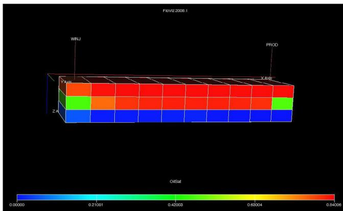
**Figure 2:** Grid block model used in simulation of asphaltene deposition.
