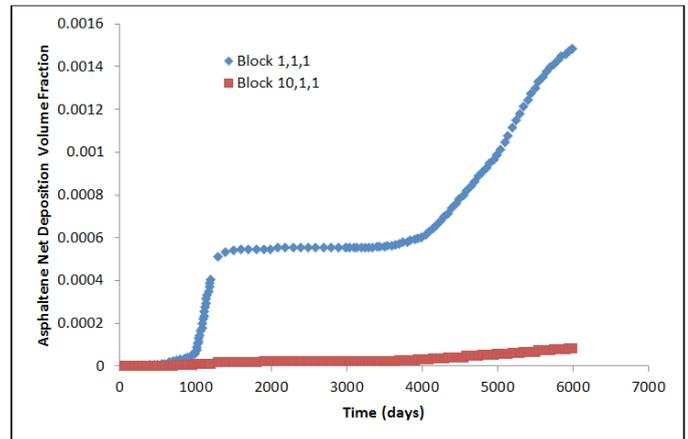
**Figure 3:** Asphaltene net deposition volume fraction vs time (days).
