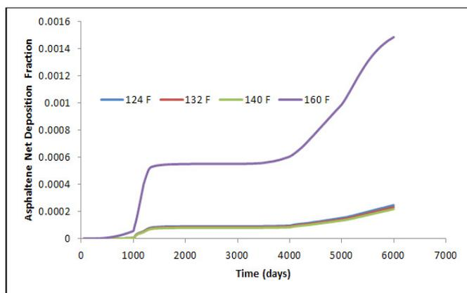
**Figure 13:** Asphaltene net deposition fraction vs time at different reservoir temperatures (injector well).
