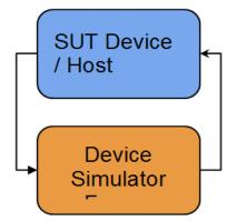
Using the mutation on the device class, the host must enumerate or restart the enumeration process once the device resets the connection. In repetition, this process would expose the software stack to issues in the enumeration area where most vulnerabilities are found. Performing such tests in the loop would make the host device more secure regarding the USB core software stack.
