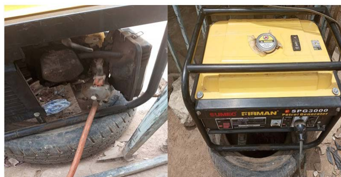
Figures 2 and 3: Small Scale Business Generator with Converted Carburetor at Auta Balefi, Karu
