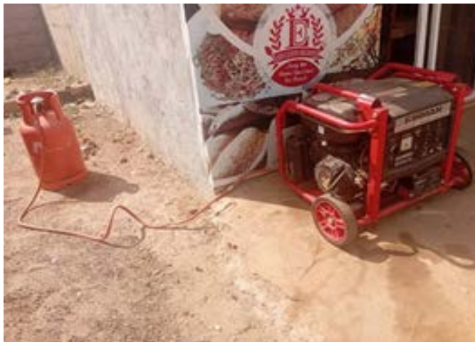
Figures 6: Converted Generator Used in Restaurant at Masaka, Karu LGA
