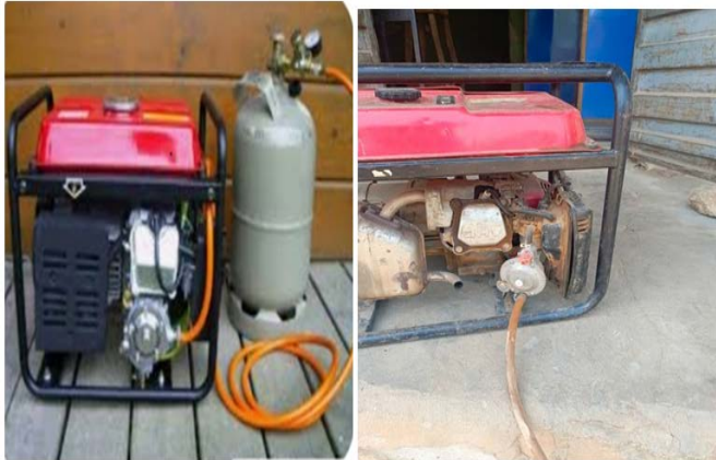
Figures 4 and 5: Converted Generator Used in Patent Medicine store and BetNija Football shop at Masaka
