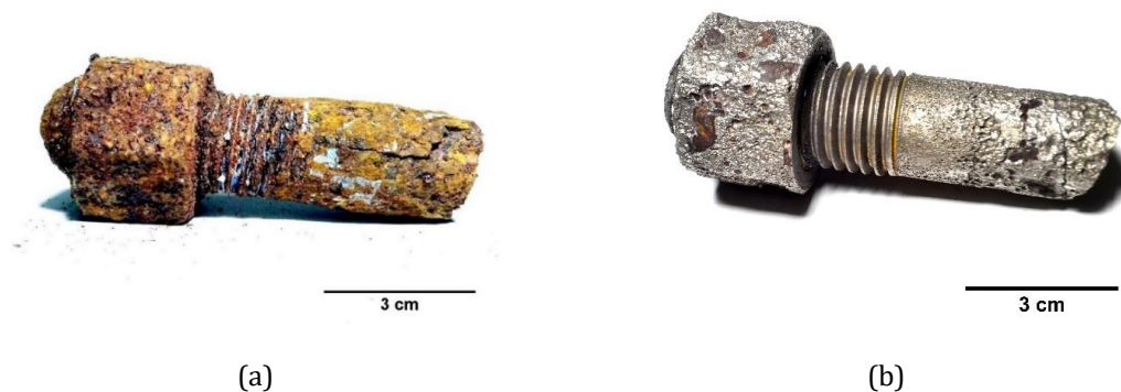
Fig. 2 Camera photographs of (a) as-received damaged and (b) as-cleaned of damaged stud bolt samples
