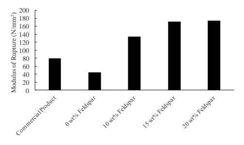
Fig. 3 Modulus of rupture of commercial and feldspar added product of Singgora
