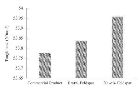
Fig. 4 Toughness of commercial and feldspar added sample of Singgora clay
