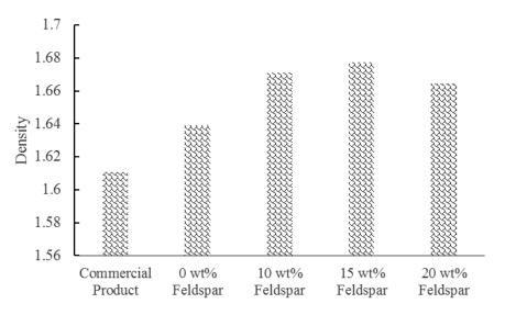
Fig. 5 Bulk density of commercial and feldspar added product of Singgora
