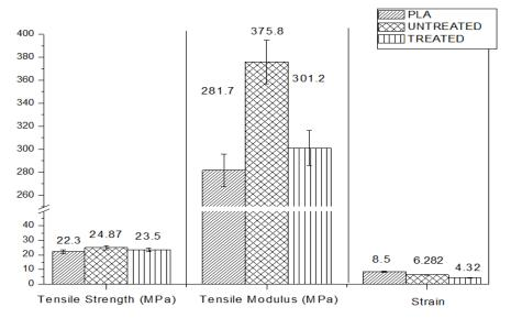
Fig. 3 Tensile strength, tensile modulus and strain for PLA, untreated PLA/DSF biocomposites and treated PLA/DSF biocomposite
