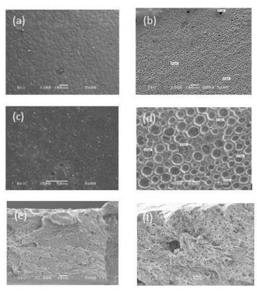
**Fig. 4** SEM migrographs of (a) and (c) untreated PLA/DSF biocomposite; (b) and (d) treated PLA/DSF biocomposites on surface at 100x magnification and SEM micrograph of (e) untreated PLA/DSF biocomposite; (f) treated PLA/DSF biocomposite on tensile fracture surface at 1000x magnification
