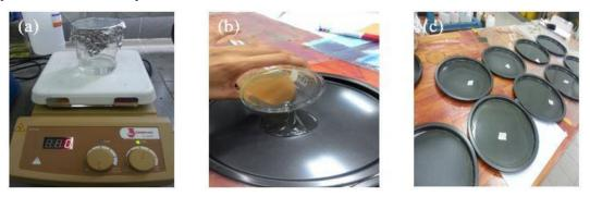
**Fig. 1** The sample preparation of PLA/DSF biocomposite films (a) stirred process with magnetic agitation on hot plate; (b) poured the sample onto flat mould and (c) left the samples for drying process
