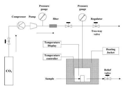
Fig. 2 The schematic diagram of supercritical carbon dioxide equipment [13]
