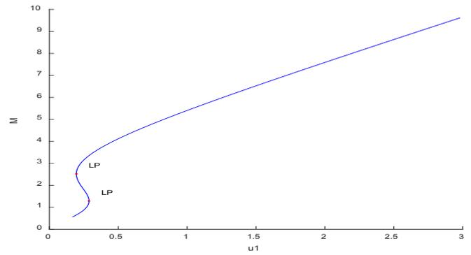
Figure 1: Limit points for model 1 when  $u_1$  was used as the bifurcation parameter.
