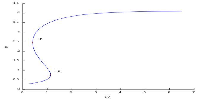
Figure 2: Limit points for model 1 when  $u_2$  was used as the bifurcation parameter.
