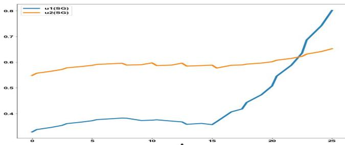
Figure 5: u1 and u2 MNL MPC profiles (model 1) with noise removed with Savitsky Golay Filter.
