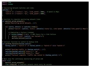
**Figure 1:** The Python script below monitors the link status and performs an automatic failover in case a link goes down.
