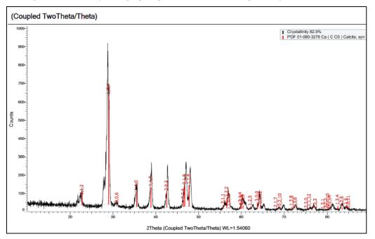
Fig. 2 X-ray diffraction pattern for the eggshell waste sample
