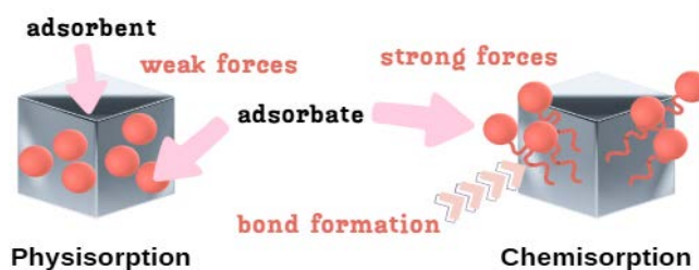
Figure 2: Graphical depiction of the difference in mechanism between physisorption and chemisorption.
