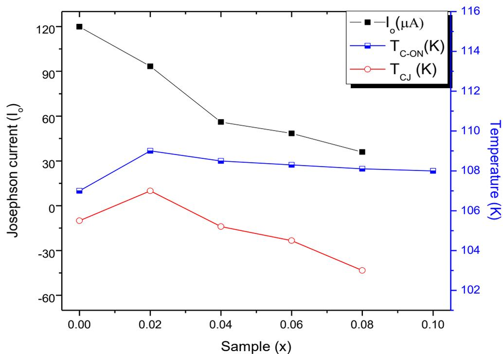
**Fig. 2** The variation of the superconducting Diamagnet ( $T_{C-ON}$ ), Phase lock-in temperature ( $T_{CJ}$ ) and Josephson current ( $I_o$ ) dependence on sample (x) wt.% of  $MgB_2$
