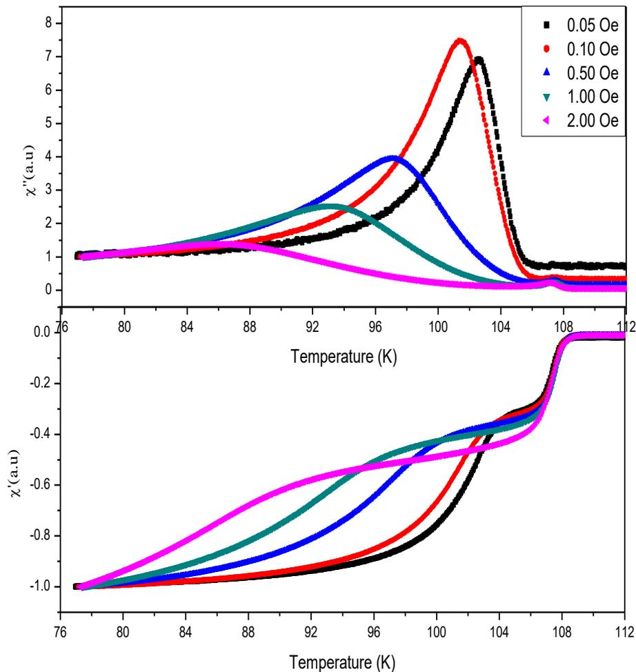
**Fig.1** Real part,  $\chi'$  and imaginary part,  $\chi''$  of susceptibility versus temperature, T at various magnetic fields for  $\text{Bi}_{1.6}\text{Pb}_{0.4}\text{Sr}_2\text{Ca}_2\text{Cu}_3\text{O}_\delta$
