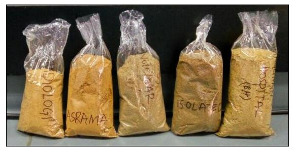
Fig. 1 Soil samples after drying process for <sup>222</sup>Rn measurements collected from six different locations
