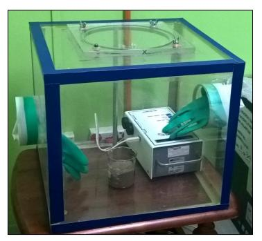
Fig. 2 Radon Sentinel 1030 monitor was used to determine <sup>222</sup>Rn concentrations level emanated from collected soil samples
